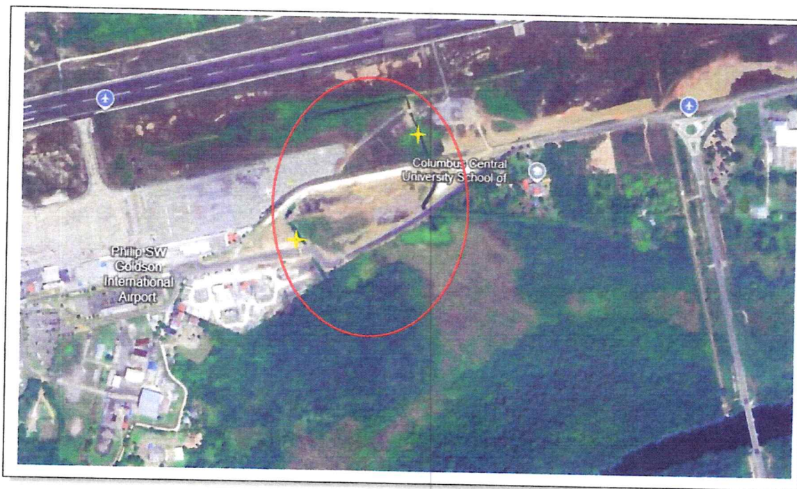
Figure – 5 Pathways for flood waters to enter PGIA facility Source: Ministry of Sustainable Development, Climate Change and Solid Waste Management
